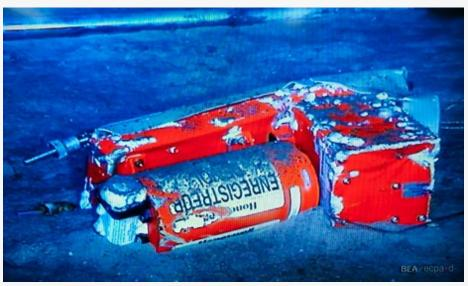
Flight Data Recorder (FDR) being recovered by a mechanical arm on the Remora 6000 Remotely Operated Vehicle; it was found *without* the Underwater Locator Beacon (ULB) chassis. Cockpit Voice Recorder (CVR) capsule with the ULB still attached, but antenna broken off.
